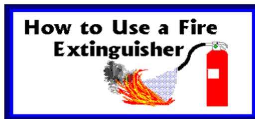
It's easy to remember how to use a fire extinguisher if you can remember the acronym PASS, which stands for Pull, Aim, Squeeze, and Sweep.
